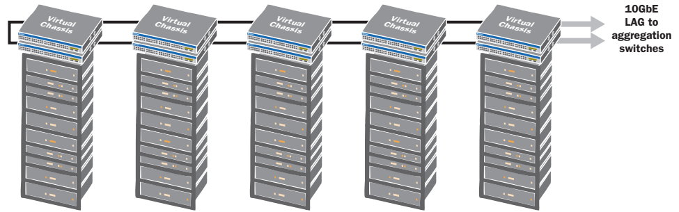
Figure 8: The Juniper EX 4200 series switches with Virtual Chassis technology reduce management overhead by creating a single managed top-of-rack device consisting of two switches each across five server racks for a total of 10 switches.
